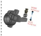
Think of bump steer as active toe when the suspension compresses or rebounds. To adjust bump steer you have to change the angle of the steering link. This is accomplished by adding or removing washers under the ball stud on the steering spindles. Anytime you change camber link locations, front arm pills, front arm spacers, or Ackermann you will need to check and possibly adjust your bumpsteer. It's best to start with zero bumpsteer or slight bump out.
