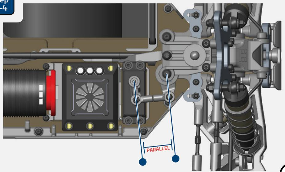
Note: Offset servo arm so it is parallel with the connecting arm at neutral or zero servo position.
