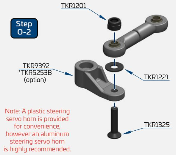
Note: A plastic steering servo horn is provided for convenience, however an aluminum steering servo horn is highly recommended.
