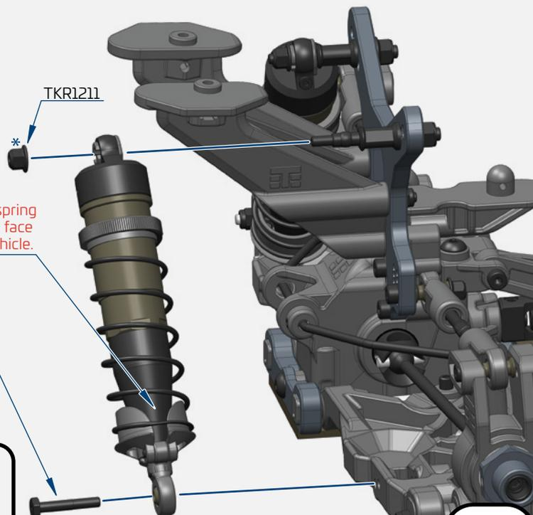
Note: Slot in spring perch should face outside of vehicle.
