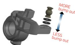
Think of bump steer as active toe when the suspension compresses or rebounds. To adjust bump steer you have to change the angle of the steering link. This is accomplished by adding or removing washers under the ball stud on the steering spindles. Anytime you change camber link locations, front arm pills, front arm spacers, or Ackermann you will need to check and possibly adjust your bumpsteer. It's best to start with zero bumpsteer or slight bump out.
