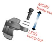
Think of bump steer as active toe when the suspension compresses or rebounds. To adjust bump steer you have to change the angle of the steering link. This is accomplished by adding or removing washers under the ball end on the steering spindles. Anytime you change camber link locations, front arm pills, front arm spacers, or Ackermann you will need to check and possibly adjust your bumpsteer. It's best to start with zero bumpsteer or slight bump out.
