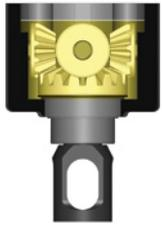
**Front:** Changing front diff oil affects overall steering response. Thinner can increase off-power steering but the vehicle may be twitchy and harder to drive. Thicker can increase on power steering and stability. We recommend 10k to 20k in the front diff.
