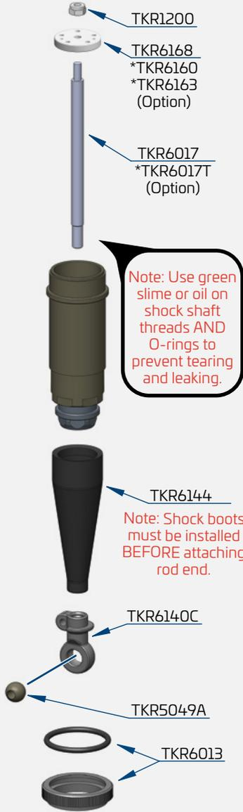
Note: Use green slime or oil on shock shaft threads AND O-rings to prevent tearing and leaking.
