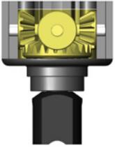
**Front:** Changing front diff oil affects overall steering response. Thinner can increase off-power steering but the vehicle may be twitchy and harder to drive. Thicker can increase on power steering and stability. We recommend 7k in the front diff.
