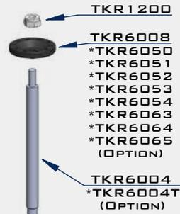
Note: Use green slime or oil on shock shaft threads AND O-rings to prevent tearing and leaking.
