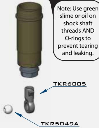
Note: Use green slime or oil on shock shaft threads AND O-rings to prevent tearing and leaking.
